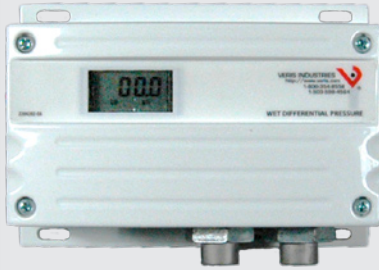
2-wire, 4-20mA pressure transducer. LCD display toggles between hi-port, low-port, and differential pressure; loop powered
